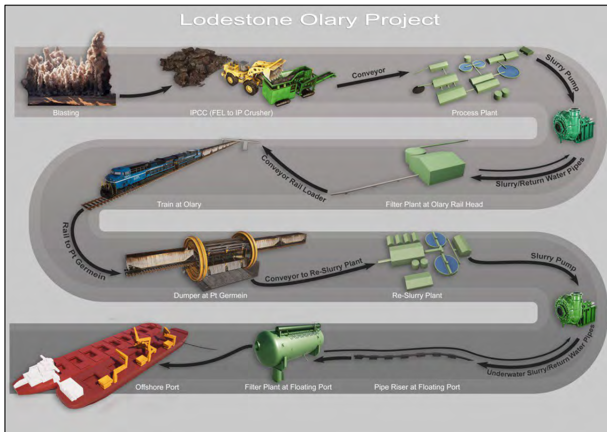
Figure 2: Conceptual production flowsheet for the Olary Project
