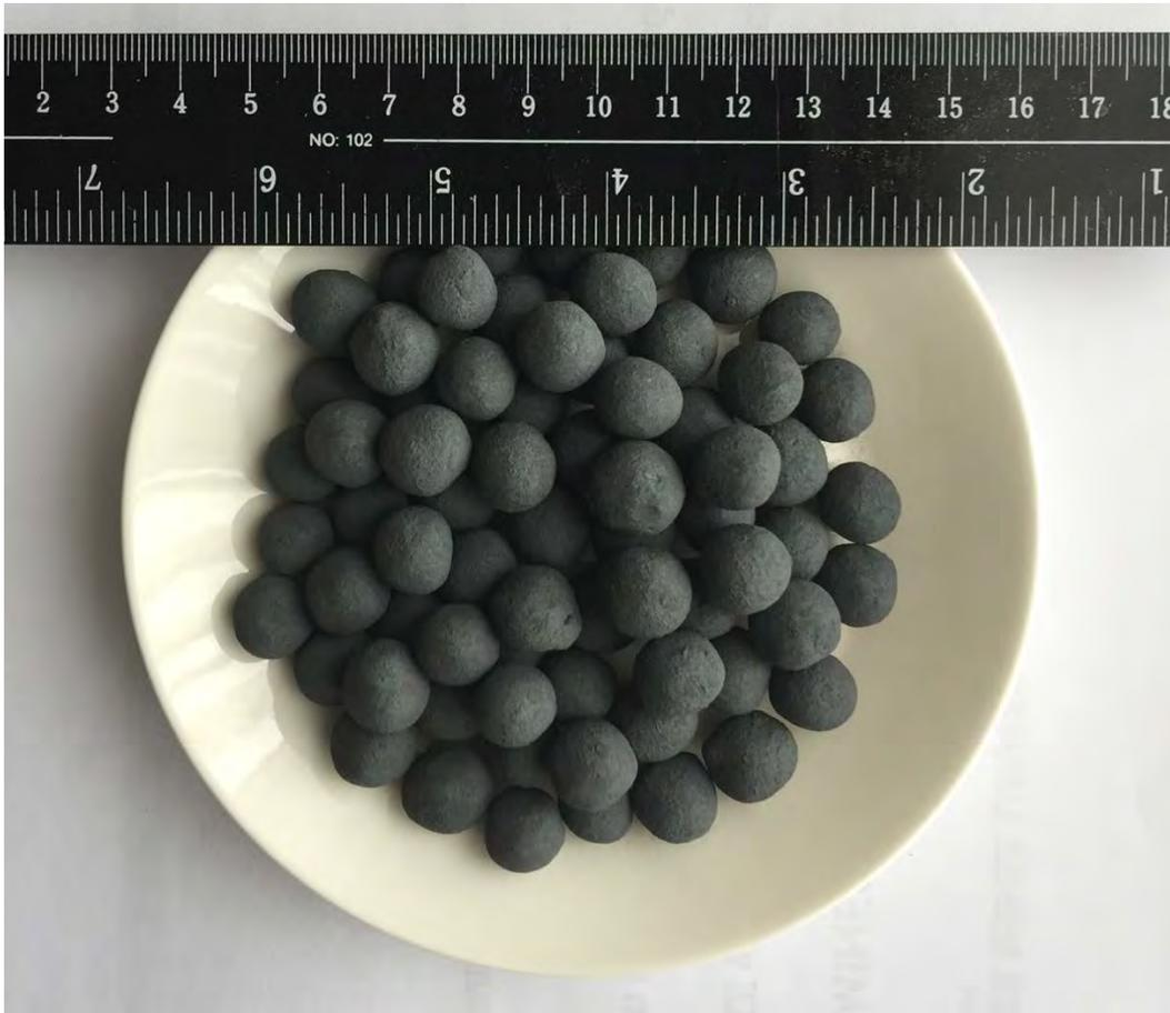
*Figure 1. Pellets made from Razorback Deposit 68% Fe concentrate*
